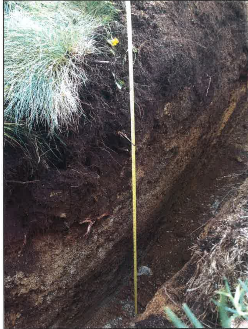
Plate 6: Test pit TP102. Test pit refusal at 1.8m on granite.
