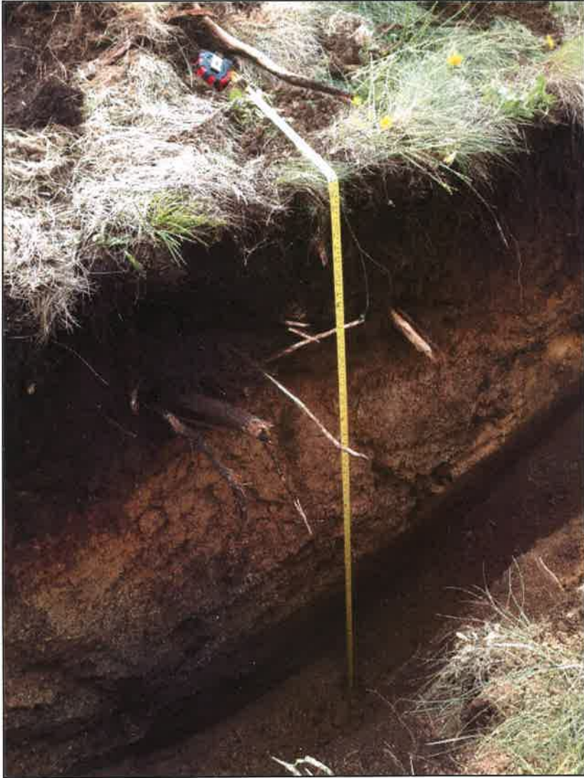
Plate 5: Test pit TP101. Test pit refusal at 2.4m on granite.
